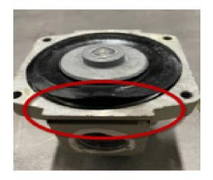
4. Remove the rear cap of the regulator to remove any tension or pressure on the diaphragm for re-assembly
