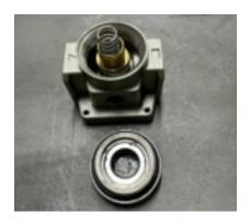
5. Ensure the diaphragm is centered and seated into the body of the regulator. Set spring on top of diaphragm
