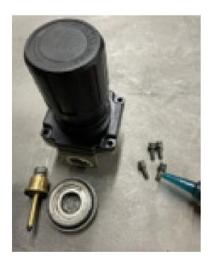
7. Reinstall the rear cap of the regulator, and reinstall the regulator to the compressor. Adjust regulator as needed for desired delivery PSI.
